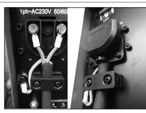
If not already connected, the connecting cable supplied must be connected to the terminals in the rear of the machine in the layout shown. The protective cover and cable clamp must be used correctly.
